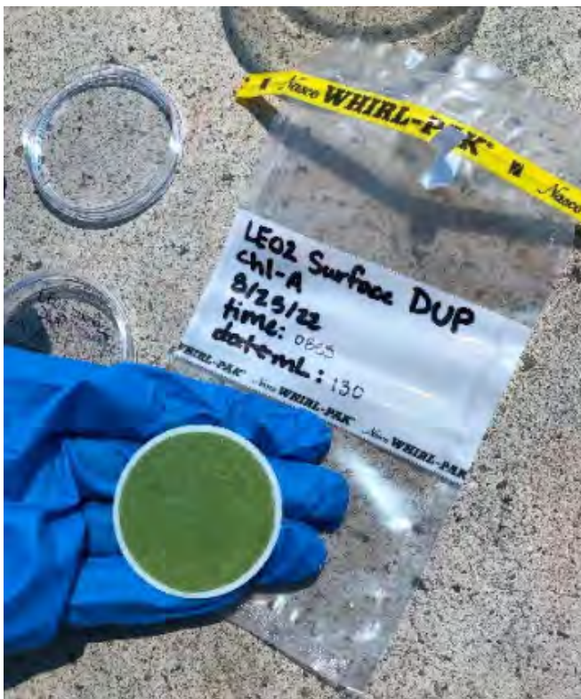
Post filtered water sample from Lake Elsinore for analysis of chlorophyll-a, a measure of algal density.
