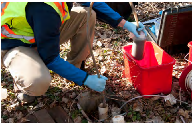
Groundwater monitoring well sampling
