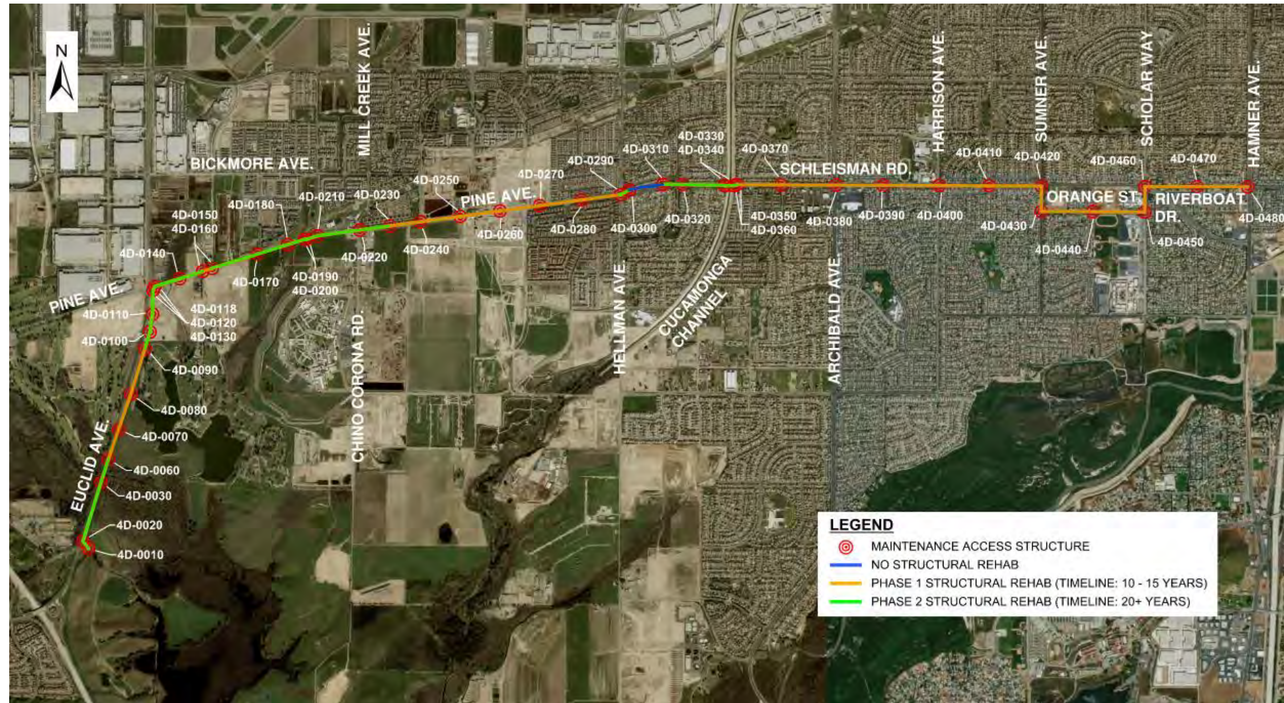
Figure 6: Reach 4D Contract 1 and 2 Alignment Segments Designated for Structural Rehabilitation in Phase 1 and Phase 2
