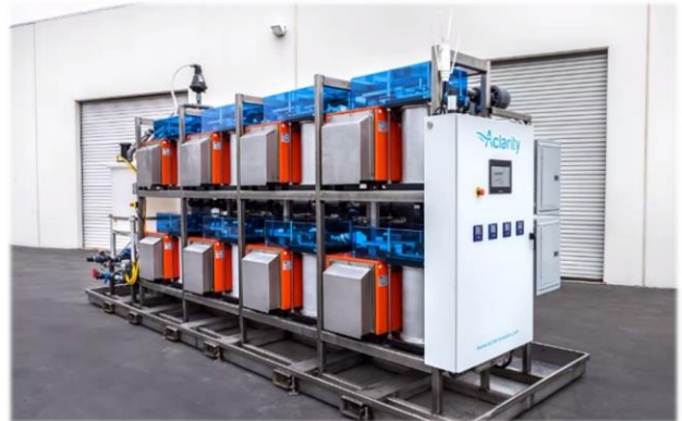
Figure 6-6 Example of EOX Treatment System (courtesy of Aclarity)
