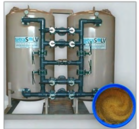
Figure 6-4 Novel Adsorbent Treatment System Example (courtesy of CycloPure)
