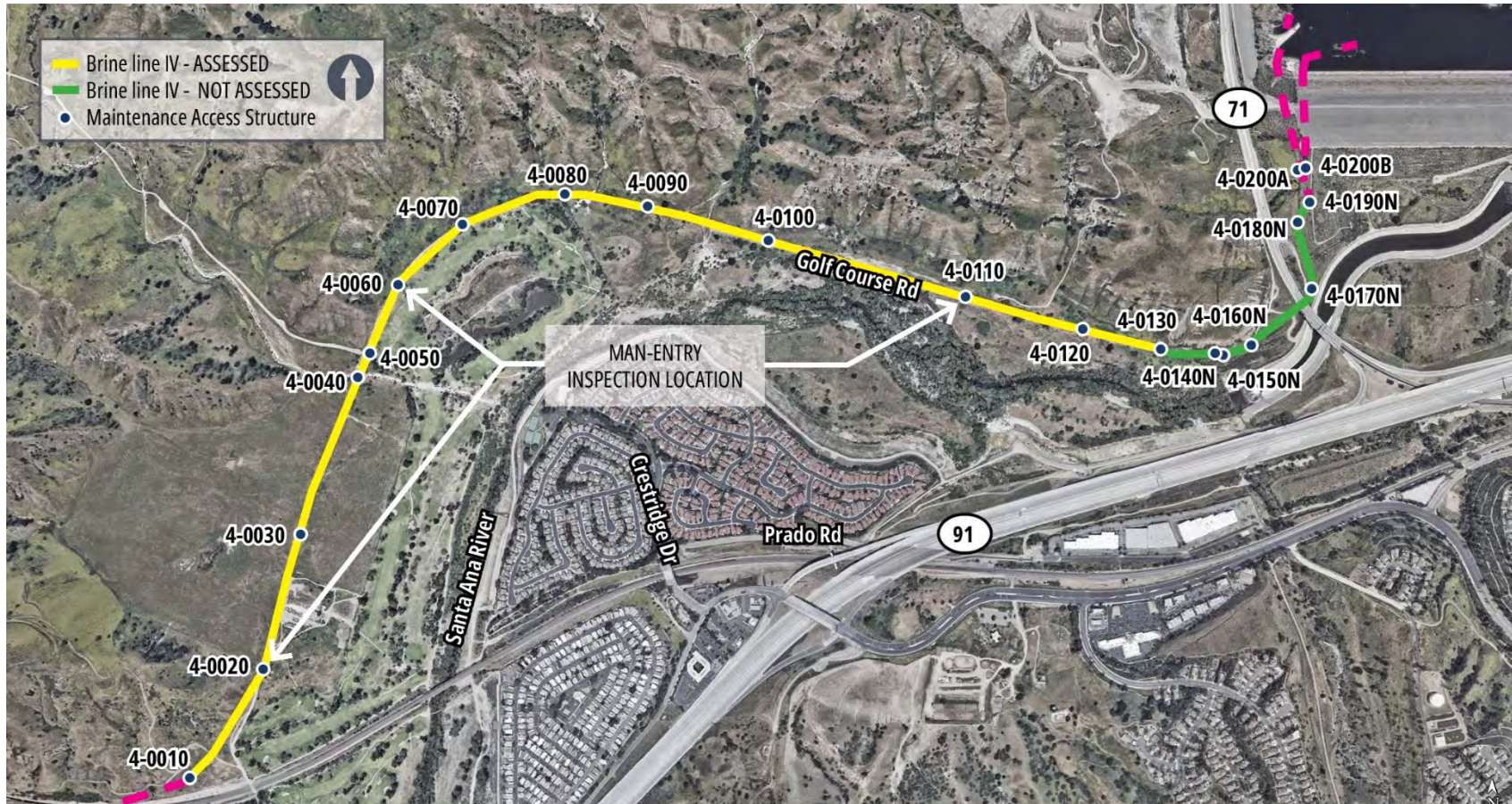
Figure 1: Reach IV Pipeline and Man-Entry Inspection Locations
