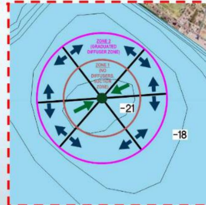
ENLARGED VIEW OF SPOKE SYSTEM
