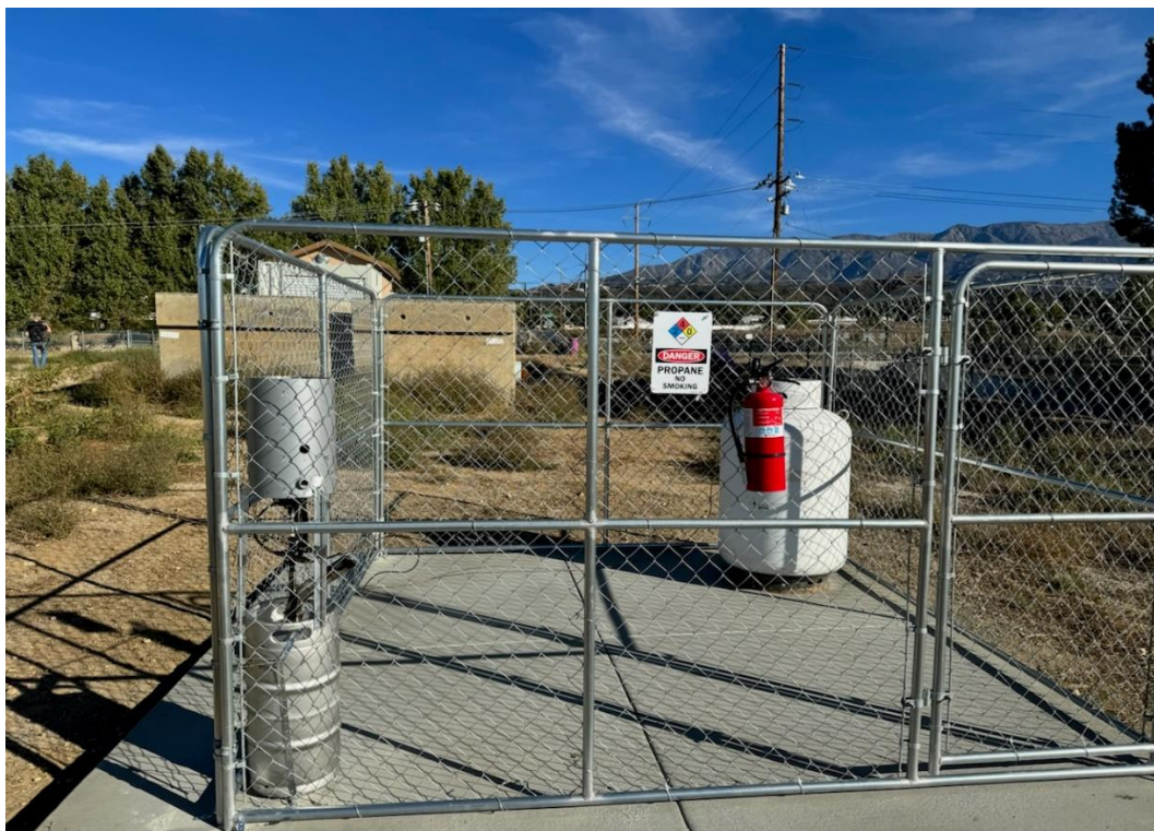
Figure 2.2. Cloud Nuclei Generator (CNG) on the left side with propane tank at site NE10.
