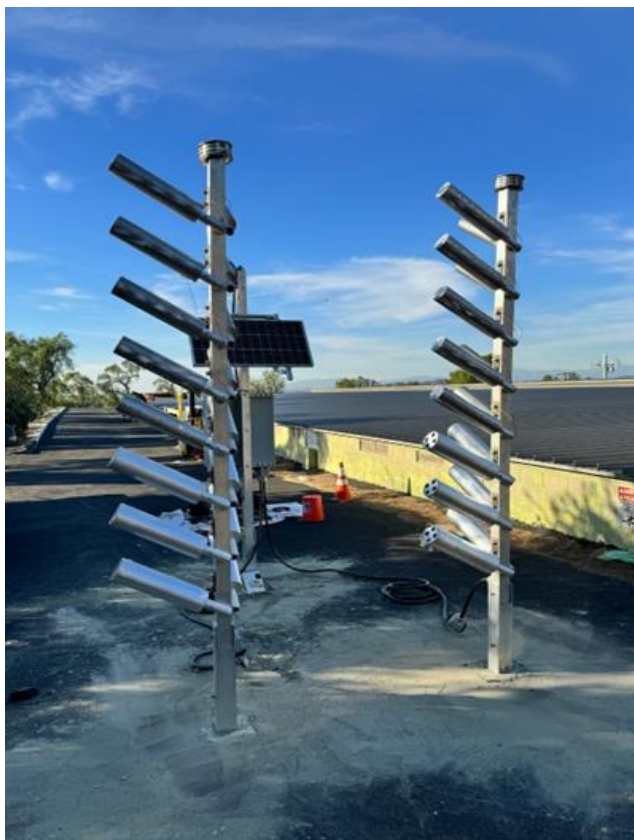
Figure 2.3. Automatic High Output Ground Seeding (AHOGS) unit located at site SW14.
