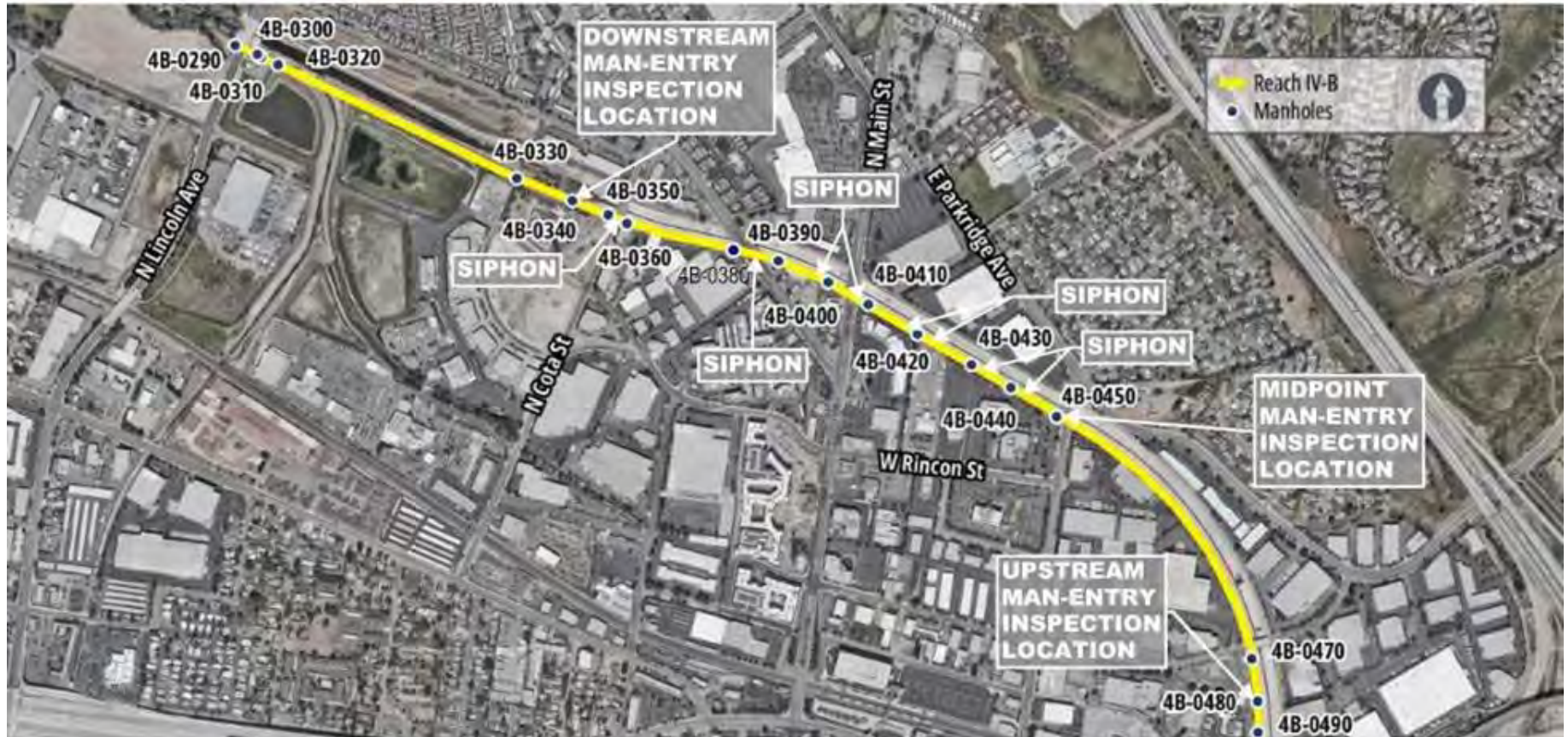
Figure 1: Reach IV-B Pipeline and Man-Entry Inspection Locations
