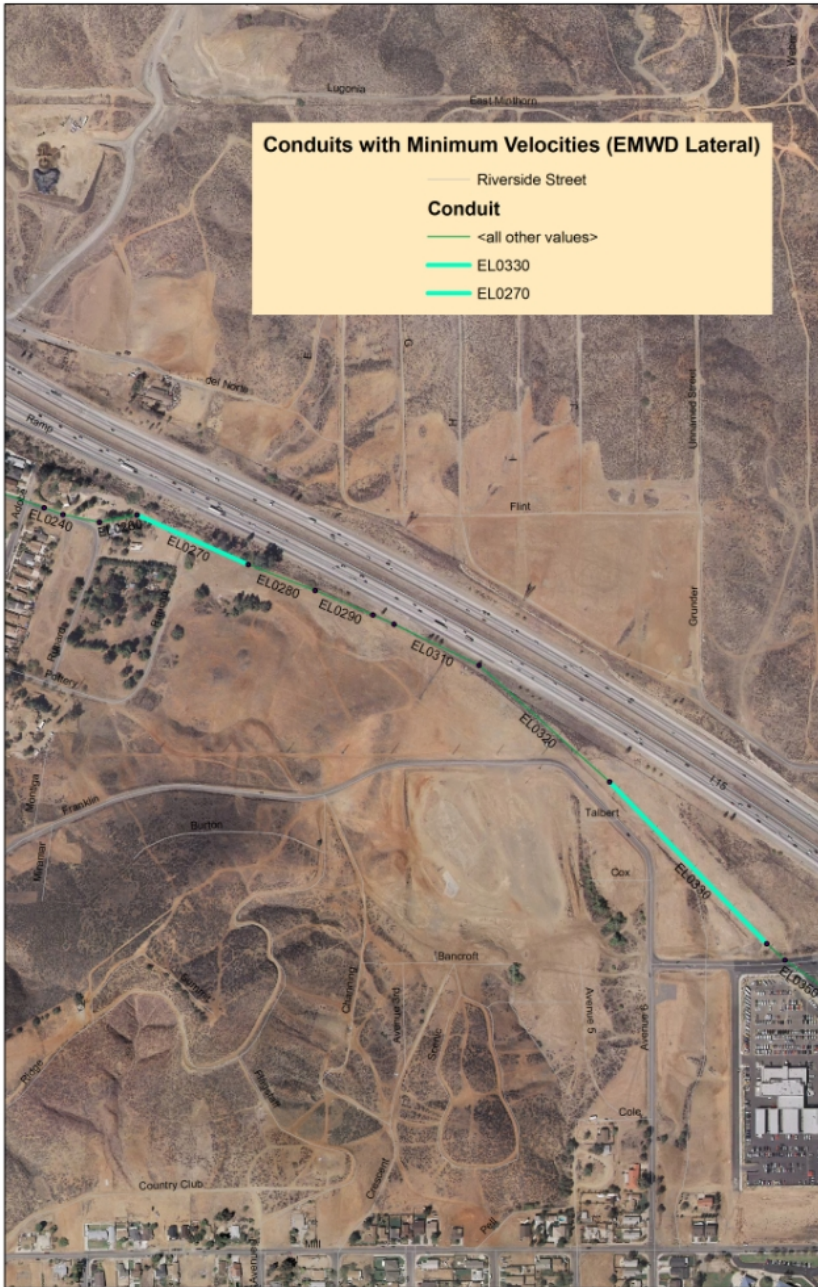
Figure A-7. Conduits with Minimum Velocity (EMWD)
