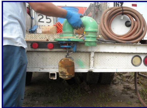
Top Flange Seat and float assembly
