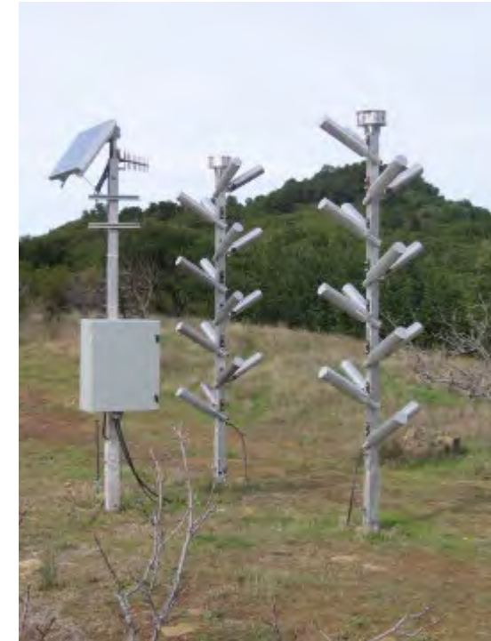
AHOGS (Automated High Output Ground Seeding Systems)
