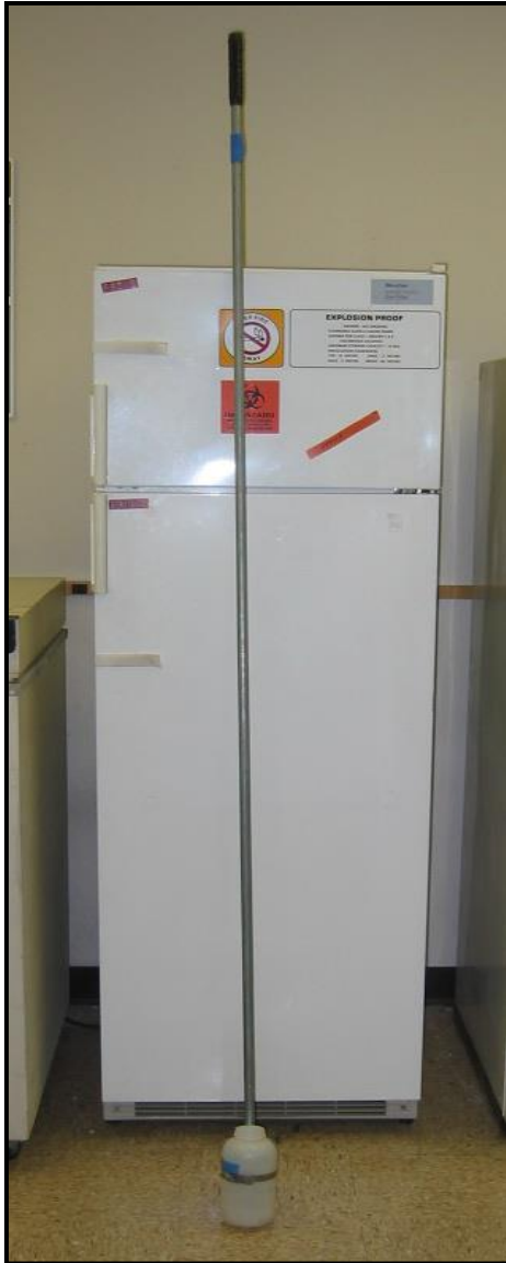
Figure 5-1. Water Sampling Pole
