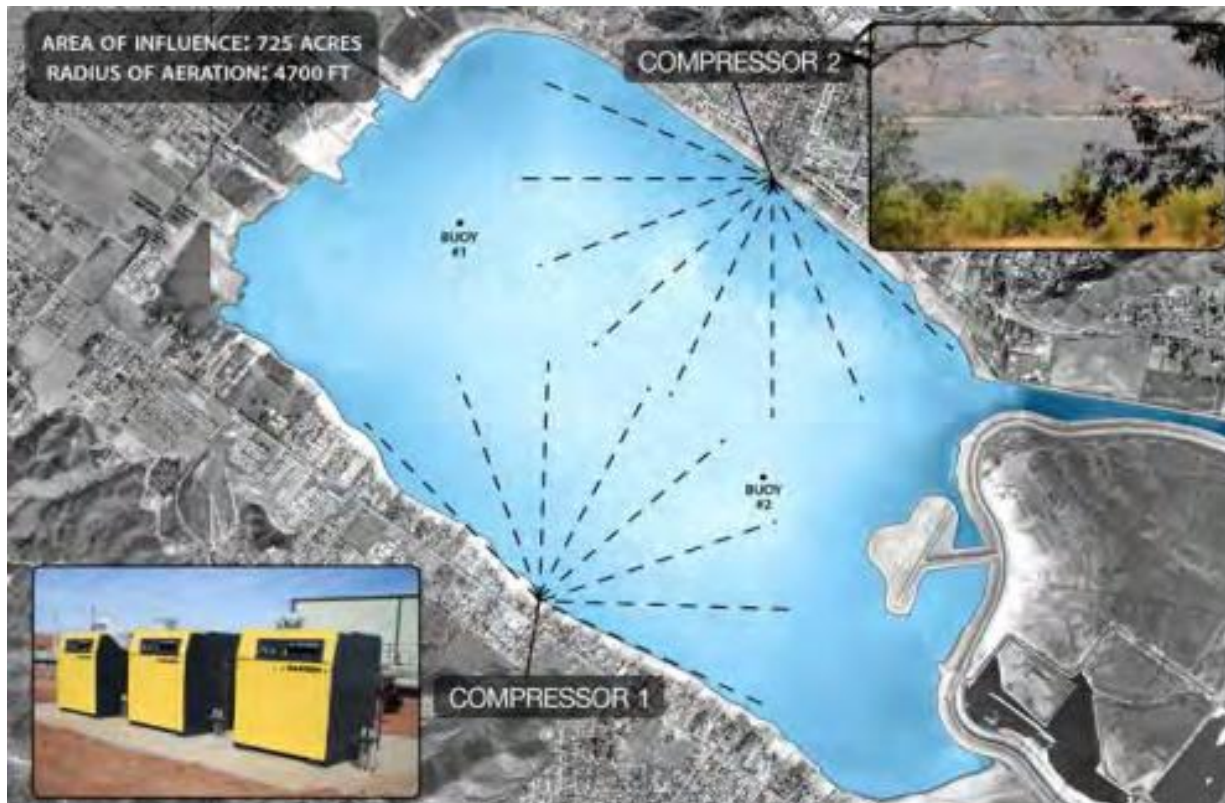
Figure 7-6. Diagram of the Lake Elsinore Aeration and Mixing System
