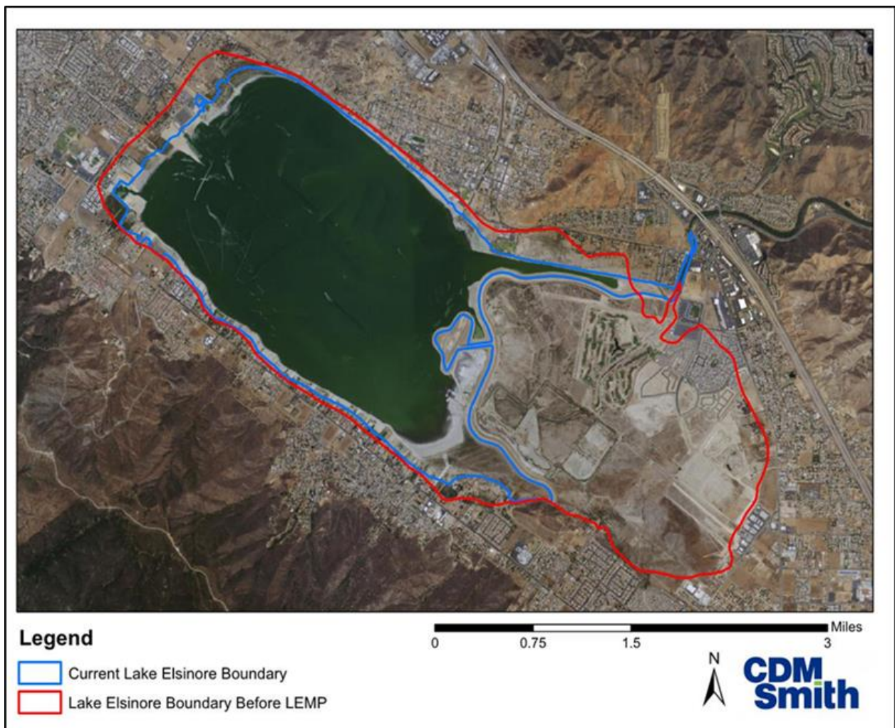
Figure 3-5. Comparison of Current Lake Elsinore Hydrography with Approximate Pre-LEMP Hydrography (shapefile from NHD)
