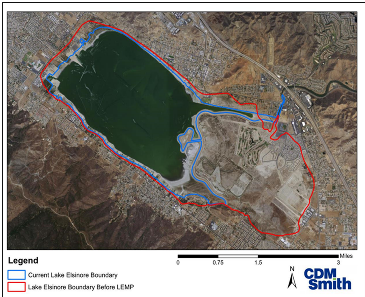
Figure 5-14. Comparison of Current Lake Elsinore Hydrography with Approximate Pre-LEMP Hydrography (shapefile from NHD)
