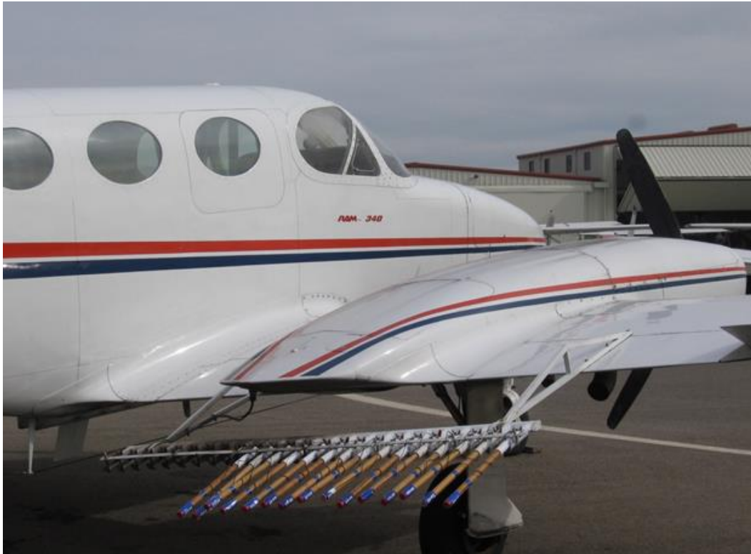
Figure 3.4. Example of a Cloud Seeding Aircraft Equipped with End Burning Silver Iodide Flares
