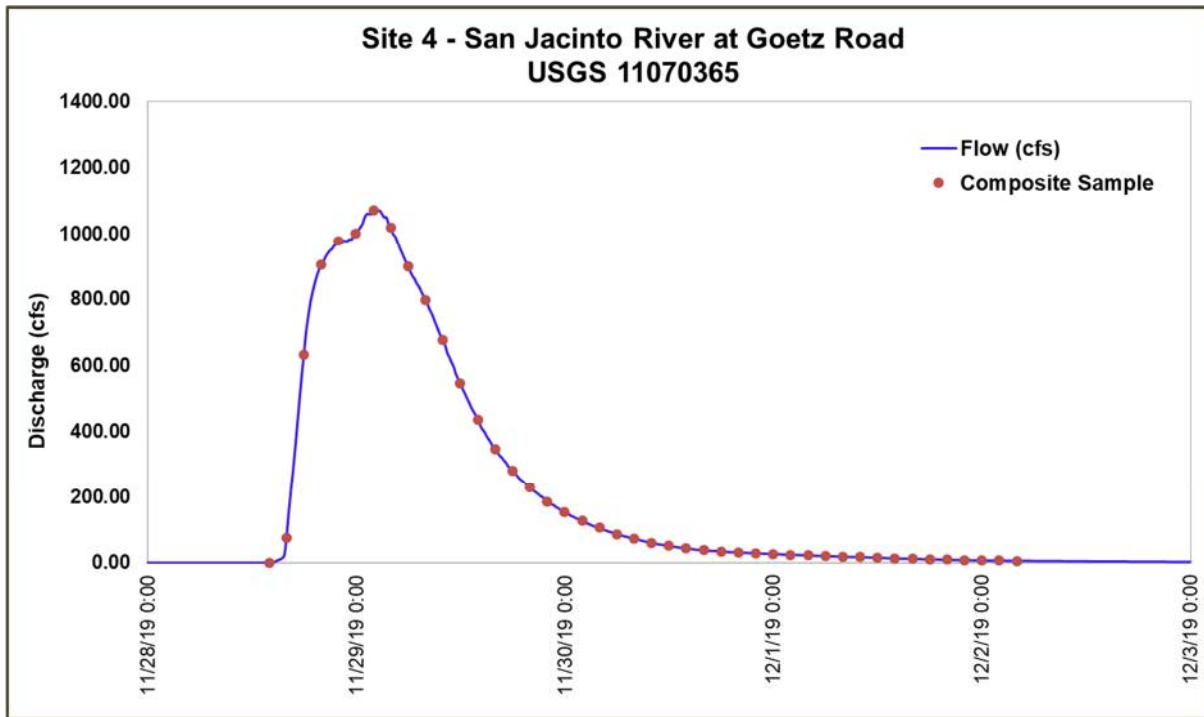
Figure 2-16. Hydrograph of First Storm Event at San Jacinto River at Goetz Road (November 28 – December 2, 2019)
