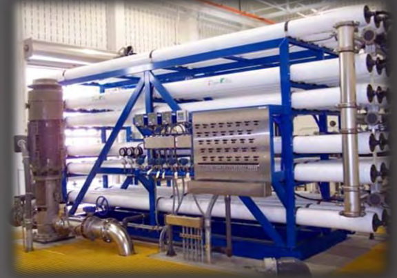
Reverse Osmosis or Nanofiltration (RO or NF)
