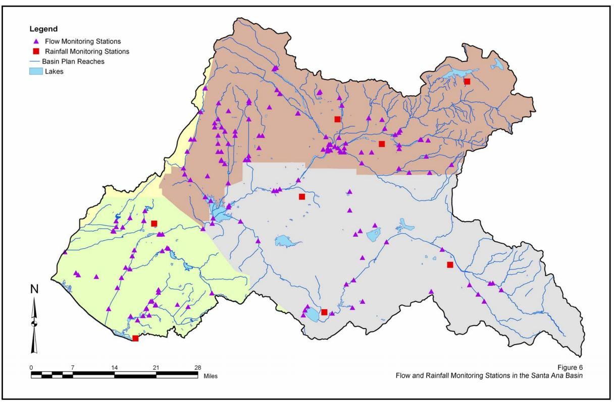
Figure 6 also shows selected long term rainfall stations located within the Santa Ana Basin that can serve as a surrogate to missing or unavailable flow data or to assess wet weather conditions for regional analyses.
