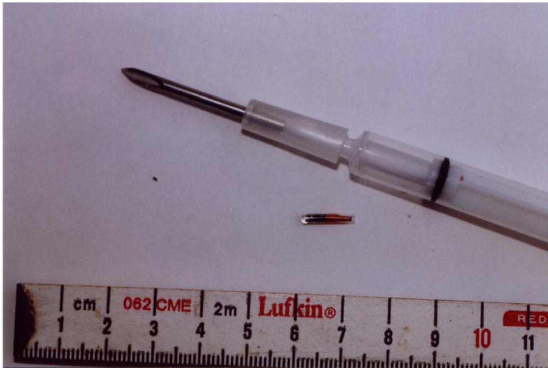
Photo 11. Close-up of PIT tag and injector needle. Notice the bevel on the injector needle. Folding meter stick provided for scale.
