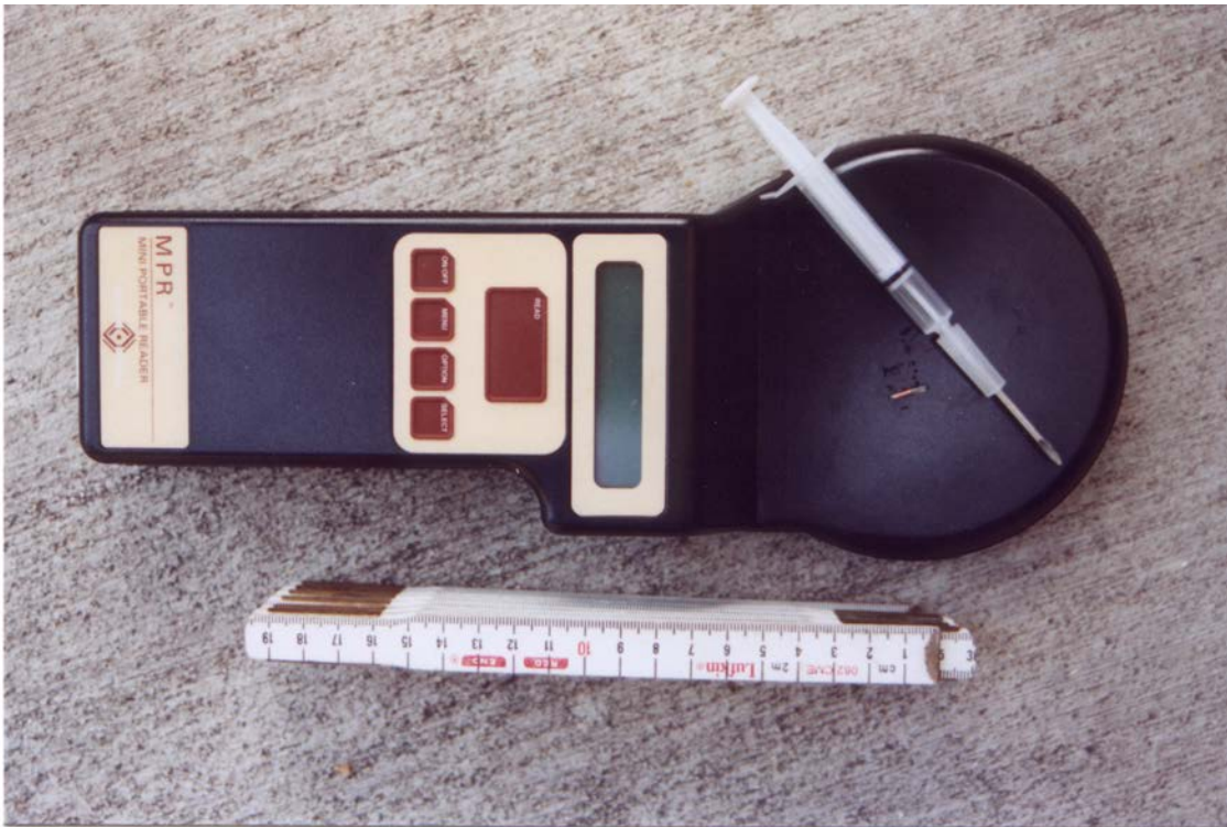
Photo 10. The PIT tagging equipment, including the reader, injector with needle and a PIT tag. Folding meter stick provided for scale.
